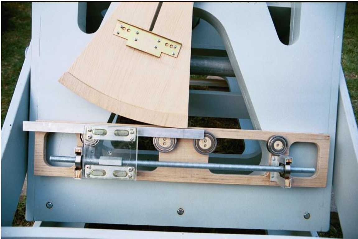
Figure 4 Using a Sector with friction instead of gearing. The driving metal section rides on a driven threaded rod – courtesy Dave Harbor, Great Plains Instruments
