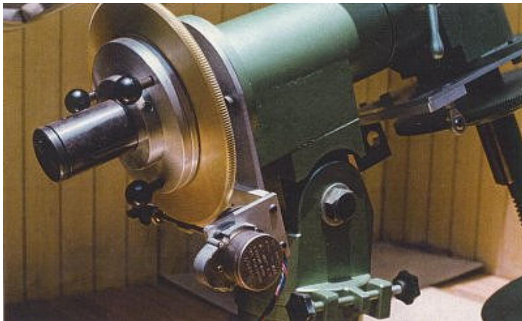
Figure 5 - Optic Craft "Polaris" Drive - capable of 95 pound load. This is a class 15 worm/gear combination. Courtesy Optic Craft.
